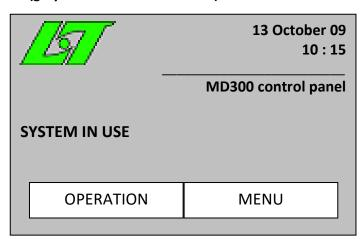
Use the function button "OPERATION" to select the screen for entering the access code
