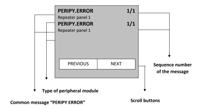
The first line of text shall include the text "PERIPY. ERROR" and the sequence number of the message. The second text line indicates the type and address of the peripheral module that caused the message. A peripheral module is an external module that is connected to the MD300 I/O bus.
