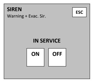
The first line shall indicate the text "SIREN". The message on the second line depends on the programming of the control panel. In the case of the standard programming, the out of service function is linked to the warning and evacuation sirens. In the event of deviating programming, only the warning sirens can be removed from service. The message on the second line is then "Warning". This manual only covers the standard programming.
