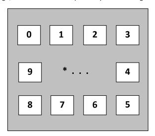
Entering a digit of the access code is suggested by "\*". If an incorrect code is entered, the system returns to the pilot screen. When entering a correct code, the system also returns to the pilot screen, but the function button "OPERATION" is colored black. The MD300 control panel is now in operating level 2.
