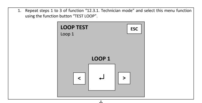
2. Select the desired detector loop using the selection buttons "<" and ">". The name of the selected detector loop is displayed in the upper left corner and in the centre of the screen. Only the actively programmed detector loops can be selected. If a detector loop has been removed from service, the text "OFF SERVICE" will be displayed instead of the loop name.
