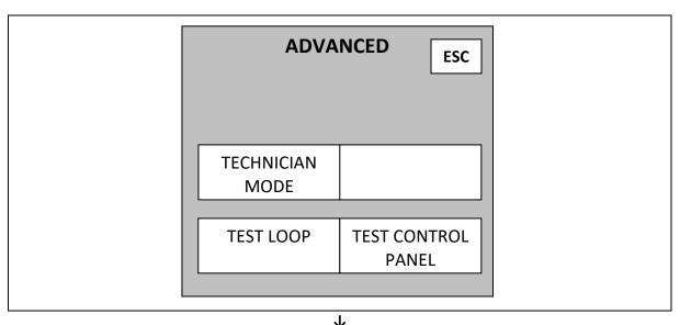
4. The current status of the technician mode is displayed in the centre of the screen. Switch the technician's mode on or off using the selection buttons "ON" or "OFF" and exit this mode using the button "ESC".
