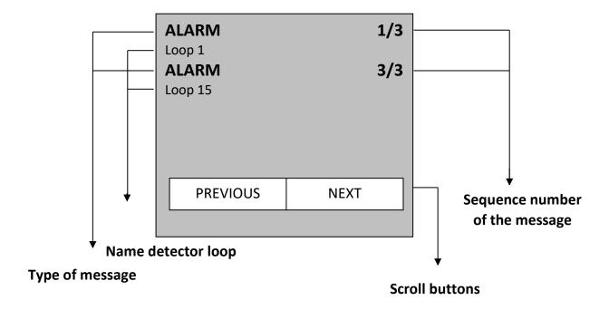
The first line of text states the type of message (e.g. ALARM) and the sequence number of the message (e.g. 1/3 is the first message out of a total of 3 messages). The second text line indicates the name of the detector loop that caused the message.
