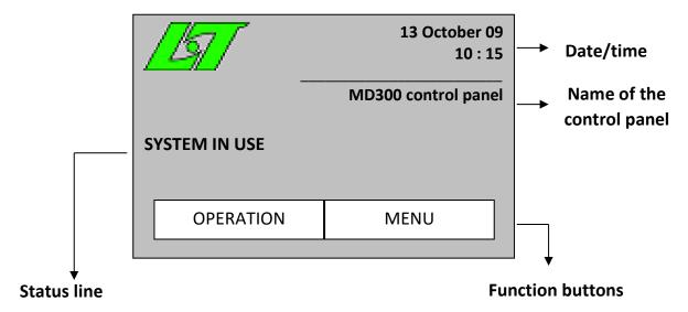
The pilot screen appears as soon as the control panel is at rest (there are no fire alarm or fault messages on the system).
