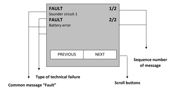
The first line of text states the text "FAULT" and the sequence number of the message (e.g.  $\frac{1}{2}$  is the first message out of a total of 2 messages). The second text line indicates the nature of the technical fault that caused the message
