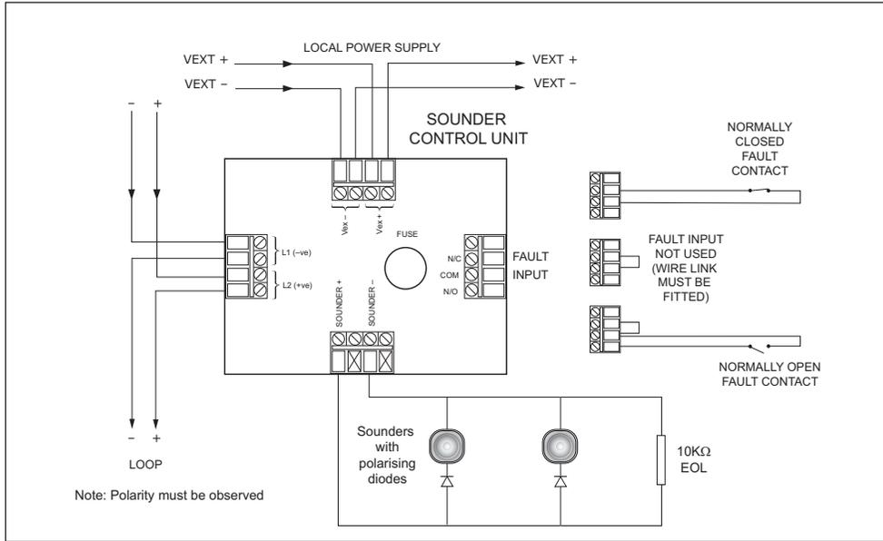
Fuse: 1.0A, anti-surge Local supply: 24V (9–32V) Sounder zone end-of-line resistor: 10KΩ, 1/3Watt
