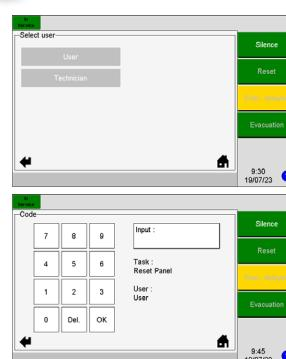
The component is now 'Out of Service'. Press the 'Reset' software button to reset the system.
