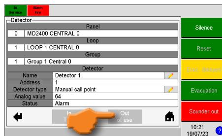
Press the 'Out of use' software button to take this component out of service.
