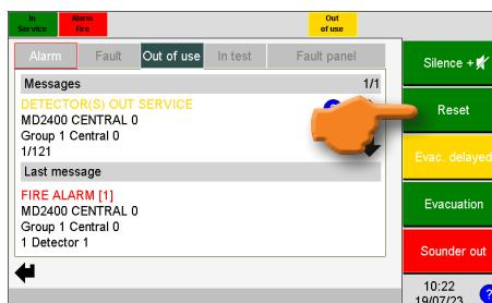
The component is now 'Out of Service'. Press the 'Reset' software button to reset the system.
