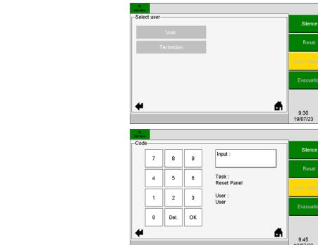
When a function requires operator mode 2 (Reset, Evacuation delayed / Evacuation immediate or Evacuation, etc.), the 'Select user' screen appears.
