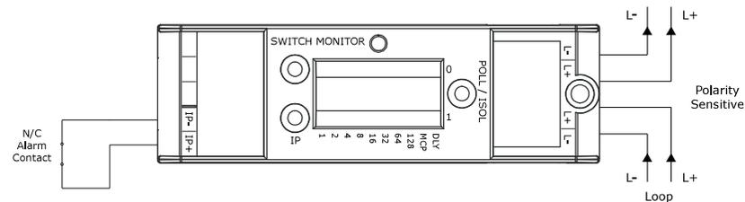
When operated under XP95 or Discovery Protocols, EN54-13 type 2 devices can be connected. In case EN54-13 type 1 devices need to be connected they must be installed directly next to this module, with no transmission path according to EN 54-13.
