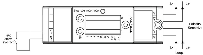
Fig. 3 N/C Monitored Circuit (Compatible with CoreProtocol only)
