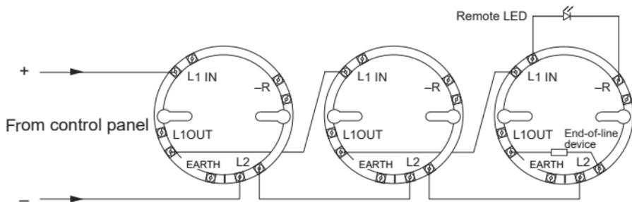
*Wiring diagram of monitored Series 65 zone*
