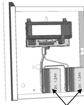
**WARNING: ALWAYS FIT 2 BATTERIES and wire in series, the product will not work with a single 12V battery**
