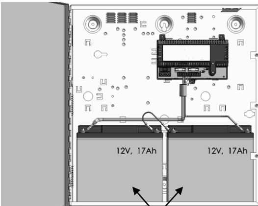
**Fit 2 x 12V 17 or 18 Ah batteries**
